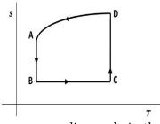
The corresponding cycle in the p - V diagram will most closely resemble
