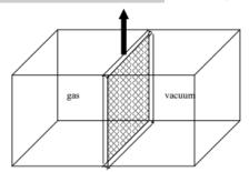
If the partition is removed and the ideal gas is allowed to expand and fill the entire container, then the entropy per molecule of the system will increase by an amount
