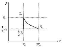
An isothermal expansion till it reaches volume  $2V_0$ , and heat Q flows into the ii) An isobaric compression back to the original volume
