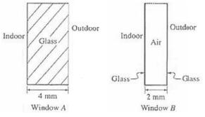
Window A is a simple pane of glass, 4 mm thick. Window B, on the other hand, consists of two extremely thin panes of glass, separated by an air gap of 2 mm, as shown in the figure above. If the thermal conductivity of glass is known to be  $0.8 \text{Wm}^{-1} \text{ K}^{-1}$  and that of air is  $0.025 \text{Wm}^{-1} \text{ K}^{-1}$ , then the ratio of heat flow  $Q_A$  through Window A to the heat flow  $Q_B$  through Window B is given by  $\frac{Q_A}{Q_B}$  =
