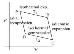
The maximum efficiency of the engine  $\eta_{max}$  is given by:
