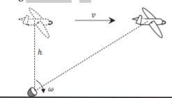
If the searchlight starts rotating with an instantaneous angular velocity  $\omega_0$  at time t=0when the plane was directly overhead, then at a later time t, its instantaneous angular velocity  $\omega(t)$  is given by
