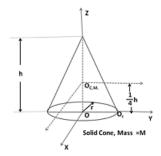
then the moment of inertia about another axis parallel to the X axis, but passing through the point  $O_r$  (see figure), is
