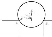
(b)  $\frac{mg}{2}$ What is the magnitude of the force exerted by point A on the disk?
