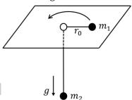
The particle of mass  $m_1$  on the plane undergoes a circular motion with radius  $r_0$  and angular momentum *L*. When a small radial displacement  $\varepsilon$  (where  $\varepsilon < r_0$  ) is applied, its radial coordinate is found to oscillate about  $r_0$ . The frequency of the oscillations is
