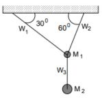
If the mass  $M_2$  is increased gradually, but without limit, we should expect the wires to break in the following order:
