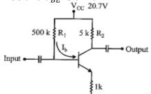
The base current  $I_B$  is (a)  $40\mu A$  (c)  $44\mu A$  (c)
