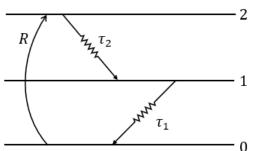
If the pump rate R is  $10^{20}$  atoms cm<sup>-3</sup> s<sup>-1</sup> and the decay routes are as shown with  $\tau_{21} = 20$  ns and  $\tau_1 = 1\mu s$ , the equilibrium populations of states 2 and 1 are, respectively, (a)  $10^{14}$  cm<sup>-3</sup> and  $2 \times 10^{12}$  cm<sup>-3</sup> (b)  $2 \times 10^{12}$  cm<sup>-3</sup> and  $10^{14}$  cm<sup>-3</sup> (c)  $2 \times 10^{12}$  cm<sup>-3</sup> and  $2 \times 10^6$  cm<sup>-3</sup> (d) zero and  $10^{20}$  cm<sup>-3</sup>.
